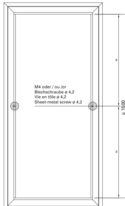
**Glazing bead fixing**
